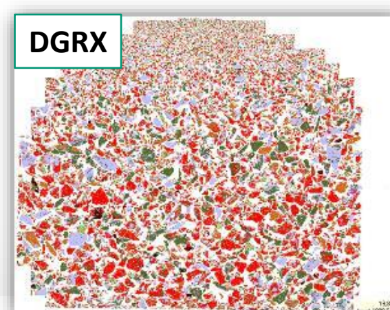
Quantitative evaluation of minerals by SEM
