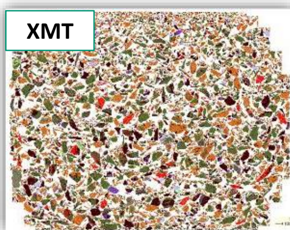
Mineralogical characterization by Qemscan
