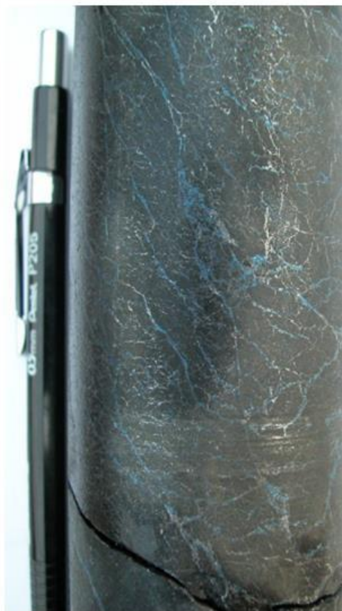
Chalcocite in stockwork
