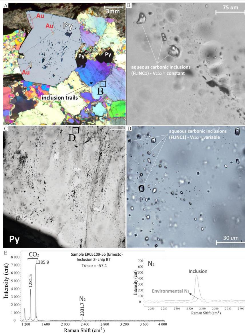
Photos of trails of aqueous-carbonic fluid inclusions in ore bearing quartz surrounding gold-bearing pyrite crystals and Laser spectroscopy showing volatiles composition
