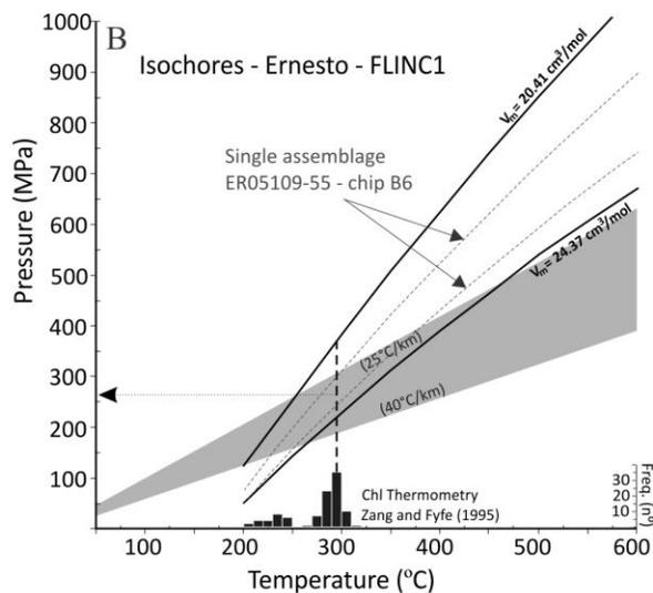
Chlorite geothermometry and calculates isochores for FLINC1
